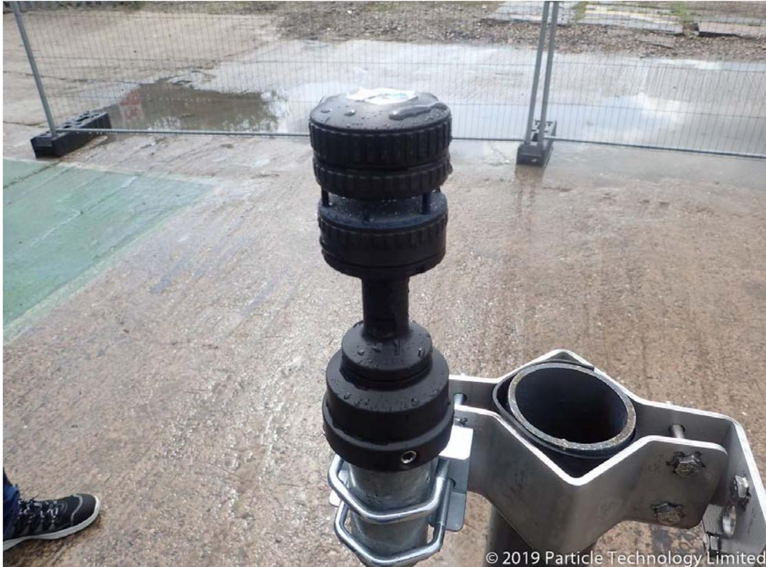
**Figure 1 – EUT in IPX6K water test area.**
