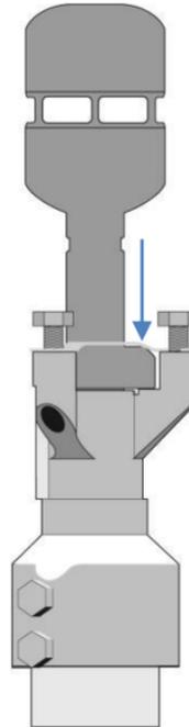
3.4 Slide the spring clip down to the base and rotate it so that it lines up under the M8 bolts (left).
