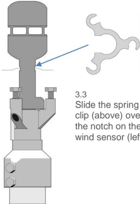
3.3 Slide the spring clip (above) over the notch on the wind sensor (left).
