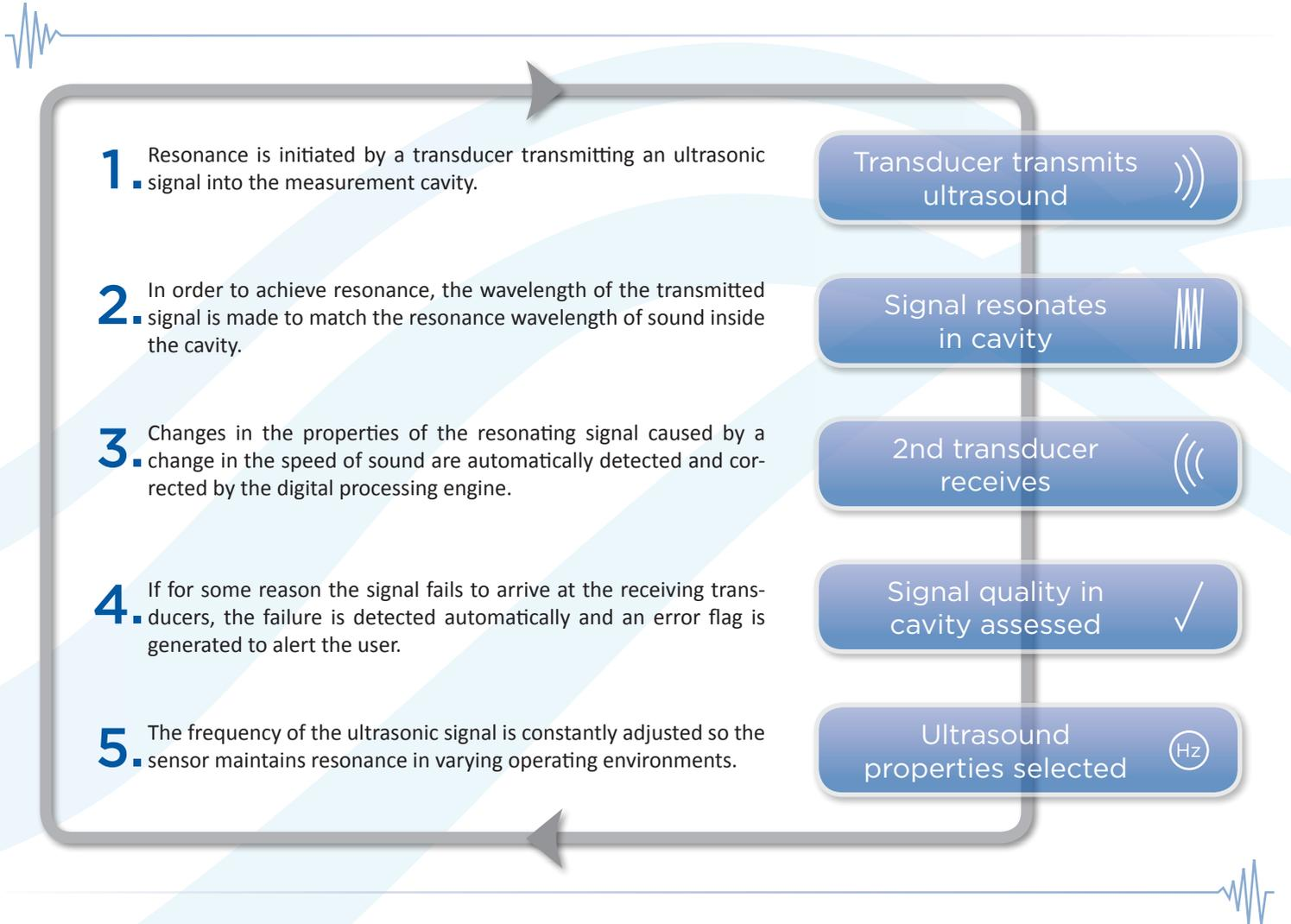
The sensor inherently compensates for changes in the air's temperature, pressure or humidity.
